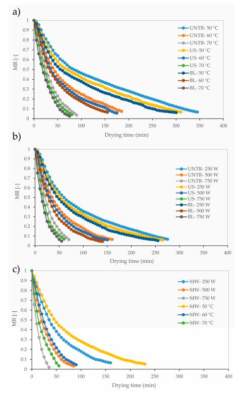
**Figure 1.** Changes in the moisture ratio of terebinth drying using ultrasound and blanching pretreatments in (**a**) convective dryer; (**b**) infrared dryer; (**c**) using microwave pretreatment in convective and infrared dryers.
